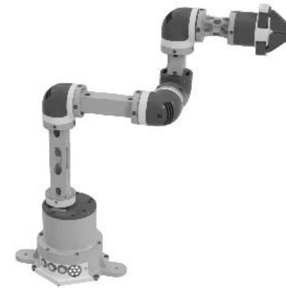
Fig. 18 Resulting low-cost lightweight robot with topology-optimized and post-processed components for n_p = 100 load cases
