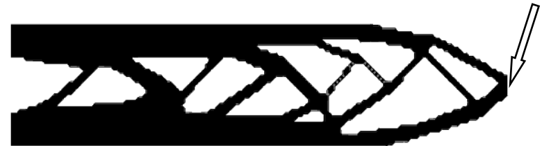
Optimal topology for single loading case ( \alpha= \alpha_0 , iterations: 150, volume: 117.1 m 3 )
