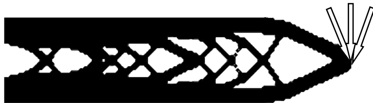
Optimal topology for multiple loading case (iterations: 123, volume: 134.2 m 3 )
