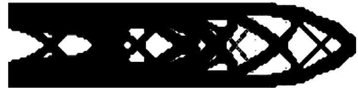
Envelope of optimal topologies for three single loading cases (volume: 154.3 m 3 )
