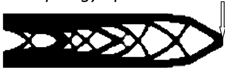
Optimal topology for single loading case ( \alpha=0 , iterations: 126, volume: 132.1 m 3 )
